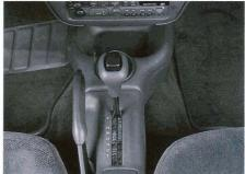
Gear indicators can be on the control panel or on the console.
